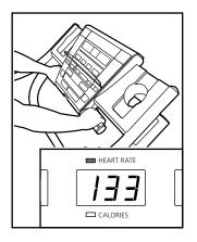
moving your hands. When your pulse is detected, the Heart Rate indicator will flash, three dashes (---) will appear in the Heart Rate/Calories display, and then your heart rate will be shown. For the most accurate heart rate reading, continue to hold the contacts for about 15 seconds.
